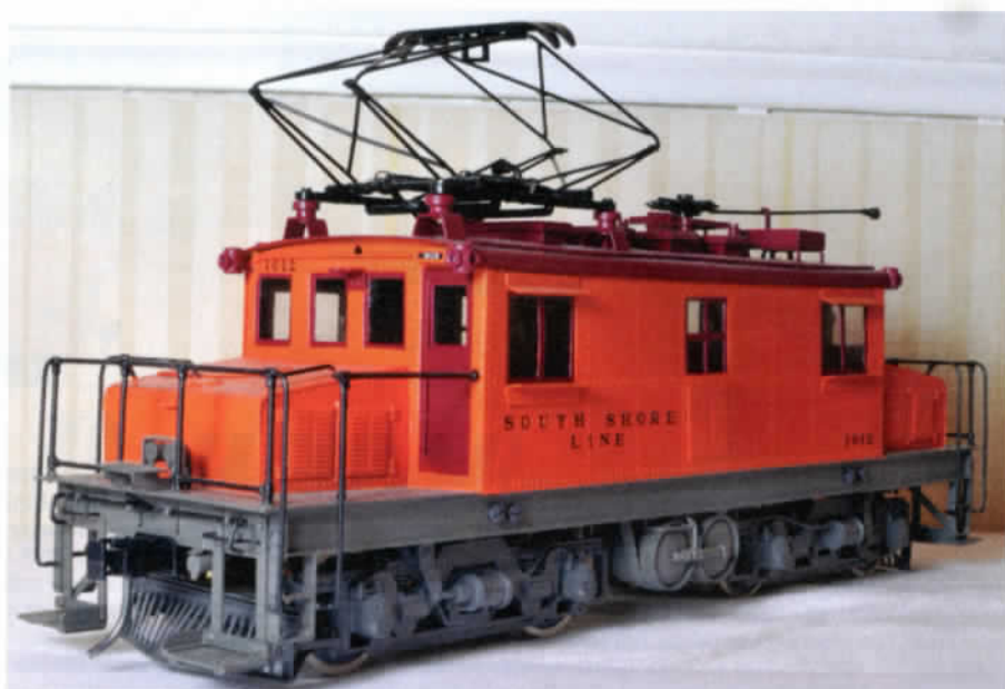
John Ainsworth's O scale South Shore electric motor—believed to be an old International Models offering from the mid-1950's—was bought for a song as a basket case. He scratchbuilt many of the detail parts, then added Micro-Mark O scale rivet decals as the model lacked any rivets ( above ). This handsome Frisco Ten-Wheeler ( below ) was among four scratchbuilt HO scale steam locomotives that John also displayed.
